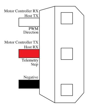
Figure 1: JR Servo Communication Connector
